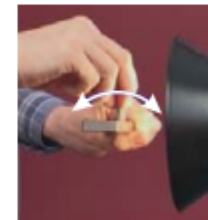
Figure 3. Visual inspection of scraper
