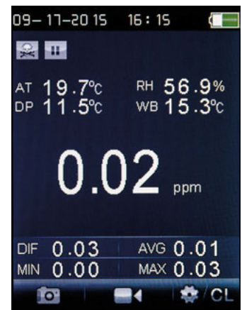
With the PC220 it is also possible to detect carbon monoxide concentrations in the air.
