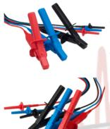
10 kV lead set Cable insulation rating: 12 kV d.c. (marked on cable) Cable type: flexible dual insulated silicon (inner insulation layer coloured white to highlight damage)
