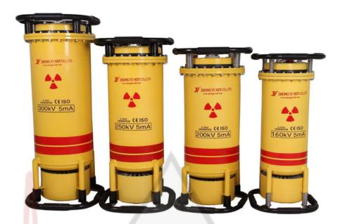
Glass Tube panoramic x ray flaw detector is made of panoramic glass tube and HV coil, which has 360 degree exposure angle; widely for circumferential weld inspection such as pipeline, boiler project inspection.
