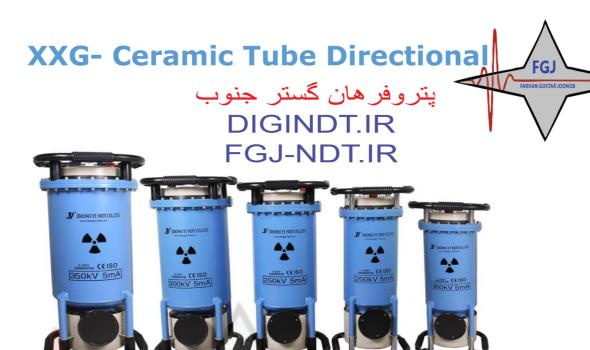
Ceramic Tube Directional X-Ray Flaw Detector is made of directional ceramic x ray tube and HV coil. It has advantage of small dimension and weight than glass tube, also working life is longer. Its model contains 160kv-350kv, max.penetration reach 70mm.
