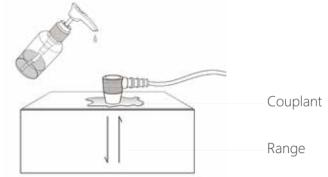
To make sure the probe working properly, it needs to use couplant to isolate the air between the probe surface and the measured workpiece surface. The liquid used for the coupling between the probe and workpiece is called as couplant.
