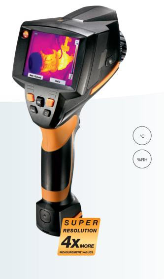
be exposed over a large area, with the thermal imager testo 875i, a single glance is enough. testo SuperResolution technology also increases the resolution of the testo 875i from 160 x 120 pixels in the Software testo IRSoft to 320 x 240 pixels. That's four times as many readings, enabling you to spot even the smallest irregularities.
