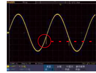
and 75,000 wfms/s refresh rate, easily capturing exceptional, and low probability events
