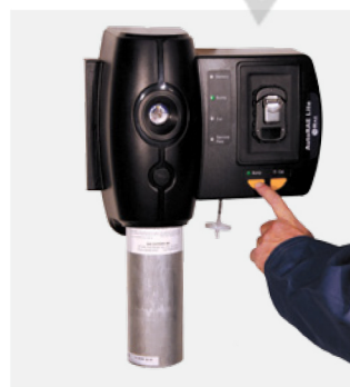
Bump testing ToxiRAE 3 with AutoRAE Lite Bump Test and Calibration Station
