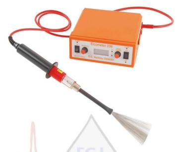
The Elcometer 236 Holiday Detector provides high voltage porosity testing to detect pits, flaws, holes, etc. in a wide variety of non-metallic coatings.
