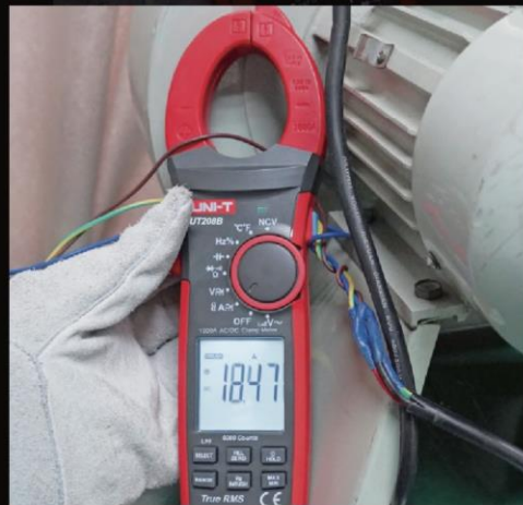
Inrush current capture (UT206B/207B/208B)
