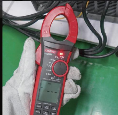
NCV Multi-Segment Display and audio/visual alarm
