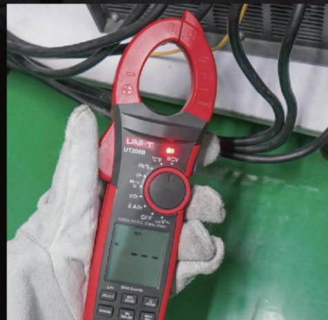
NCV Multi-Segment Display and audio/visual alarm
