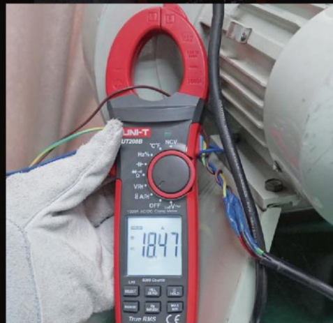
Inrush current capture (UT206B/207B/208B)
