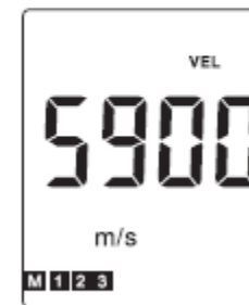
Last applied sound velocity & registered unit
