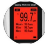
Red backlight indication when alarm happen
