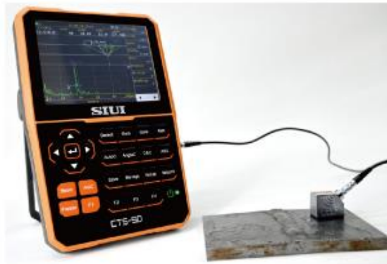
UT inspection for butt weld
