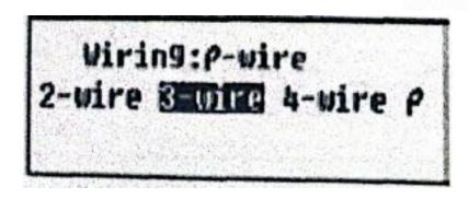
Select the appropriate Wiring System with the Cursor Key and press the <u>ENTER/SAVE</u> Key. Then the CONFIG\_SETTING Screen with the selected Wiring System will be displayed.
