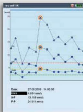
Recording of overall velocity signals, RMS, 0-p and p-p.
