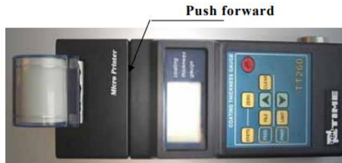
Fig. 5-3 installation and dismantle of printing head
