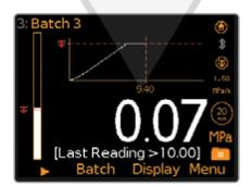
Either pull to maximum or pull to preset limit. Unique time hold feature allows users to set a delay before pressure returns to
