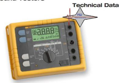
rod and each are connected to the tester. No earth ground stakes are used at all. A known, fixed voltage is induced by one clamp and the current is measured using the second clamp. Then the tester automatically determines the resistance of the earth ground rod.
